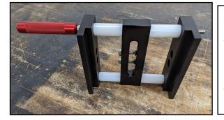
4. Slide the chainsaw bar through the black center guide. There are gripper teeth to hold the bar stationary.
