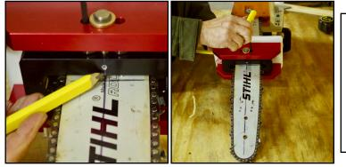
3. Center the tool on the bar as shown at left, and tighten the set screws alternately with the 3/16 T-wrench provided. Using an open end 9/16 wrench, tighten the lock nuts.
