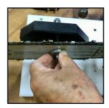
1. Drill a 3/8" hole in your chain saw bar. Center hole in the middle of the bar, approximately 4" from the motor.
