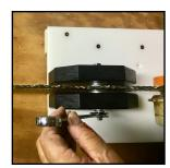
3. Unscrew the nut from the end of the bolt and remove (2) washers. Mount chainsaw in EZ Slotter and add the (2) washers that you previously removed so there are (2) on each side of the bar.
