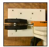
4. Replace block by reinstalling the (3) screws in the bottom of the EZ Slotter. Tighten the nut so bar is snug but moves freely.
